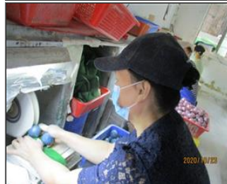
Photo of non-conformity NC 7.6 Inappropriate PPE wearing.JPG
