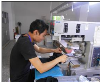
Photo of non-conformity NC 7.6 Worker not wear glove or mask.JPG
