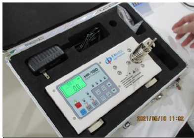
Description:Torque control for electric screwdriver.
