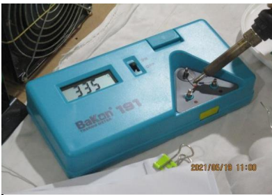
Description:Temperature control for soldering iron
