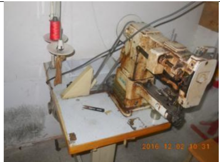
No pulley guard was installed for 2 out 8 sewing machines
