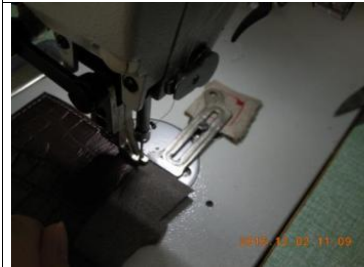
No needle guard was installed for 3 out of 8 sewing machines
