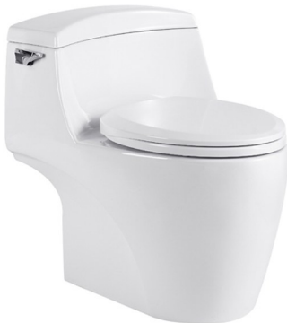
DA8088 虹吸连体坐便器 Siphonic One-piece Toilet Size: 730x450x645mm S-trap, 300mm Roughing-in 地排污口中心离墙300mm
