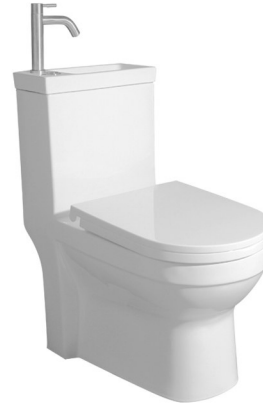
DA8304 虹吸/直冲连体坐便器 Siphonic/Washdown One-piece Toilet Size:720x370x775mm S-trap,250,300,400mm Roughing-in 地排污口中心离墙250,300,400mm P-trap,180mm Roughing-in 横排污口中心离地180mm
