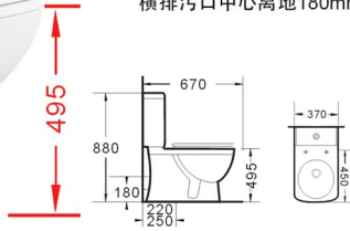
DT8040H 直冲分体坐便器 Washdown Close-couched Closet Size:670x370x880mm S-trap,220,250mm Roughing-in 地排污口中心离墙220,250mm P-trap,180mm Roughing-in 横排污口中心离地180mm
