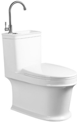
DA8302 虹吸连体坐便器 Siphonic One-piece Toilet Size:700x385x780mm S-trap,300,400mm Roughing-in 地排污口中心离墙300,400mm
