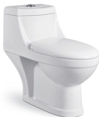
DA8018 直冲连体坐便器 Washdown One-piece Toilet Size:710x365x650mm S-trap,250,300mm Roughing-in 地排污口中心离墙250,300mm P-trap,180mm Roughing-in 横排污口中心离地180mm
