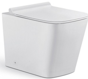
DG151-F 直冲式落地坐便器 Washdown Close-couched Toilet Size:590x350x410mm P-trap,180mm Roughing-in 横排污口中心离地180mm
