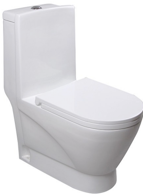
DA8073 虹吸/直冲连体坐便器 Siphonic/Washdown One-piece Toilet Size: 720x380x830mm S-trap, 250, 300, 400mm Roughing-in 地排污口中心离墙250, 300, 400mm P-trap, 180mm Roughing-in 横排污口中心离地180mm
