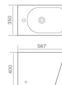
DF051 妇洗器 Bidet Size:567x350x400mm Fixing to wall with back 背靠墙式安装
