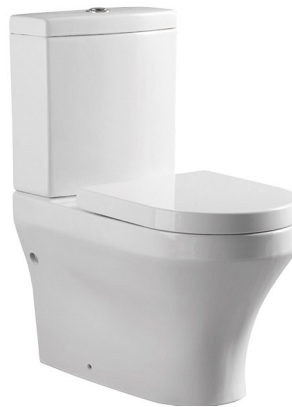
DT2512 直冲分体坐便器 WaterMark Washdown Close-couched Closet Size:640x360x800mm P-trap,180mm Roughing-in 横排污口中心离地180mm
