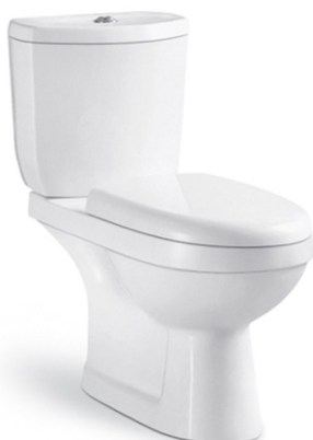
DT2020 直冲分体坐便器 Washdown Close-couched Closet Size:700x380x740mm S-trap,250,300mm Roughing-in 地排污口中心离墙250,300mm P-trap,180mm Roughing-in 横排污口中心离地180mm
