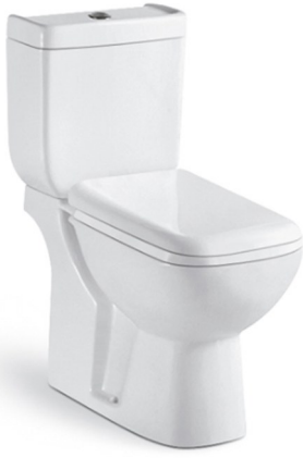
DT2040 直冲分体坐便器 Washdown Close-couched Closet Size:650x370x785mm S-trap,250mm Roughing-in 地排污口中心离墙250mm P-trap,180mm Roughing-in 横排污口中心离地180mm
