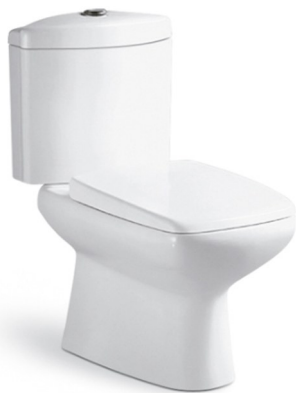
DT2044 直冲分体坐便器 Washdown Close-couched Closet Size:710x390x765mm S-trap,250mm Roughing-in 地排污口中心离墙250mm P-trap,180mm Roughing-in 横排污口中心离地180mm
