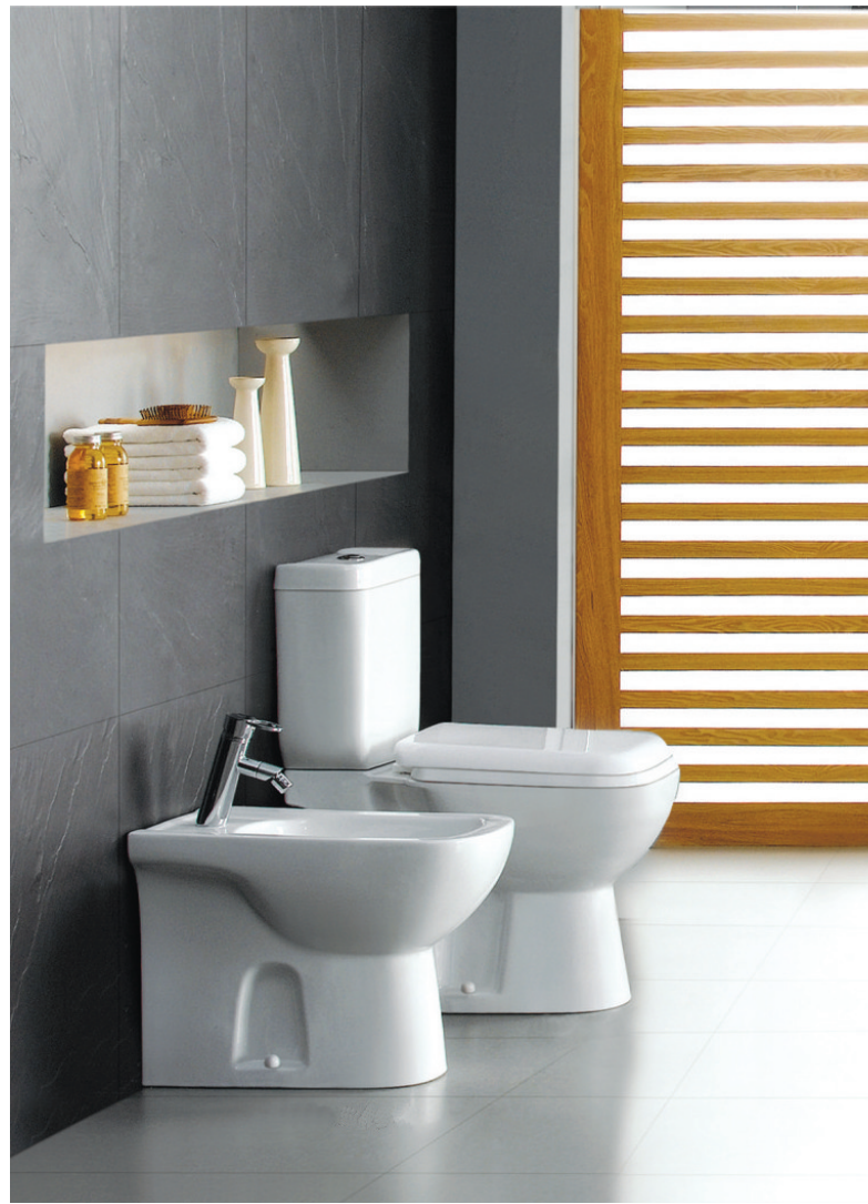
DT2040 直冲分体坐便器 Washdown Close-couched Closet Size:650x370x785mm S-trap,250mm Roughing-in 地排污口中心离墙250mm P-trap,180mm Roughing-in 横排污口中心离地180mm
