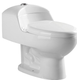
DA8015 虹吸连体坐便器 Siphonic One-piece Toilet Size:660x420x590mm S-trap,250,305mm Roughing-in 地排污口中心离墙250,305mm
