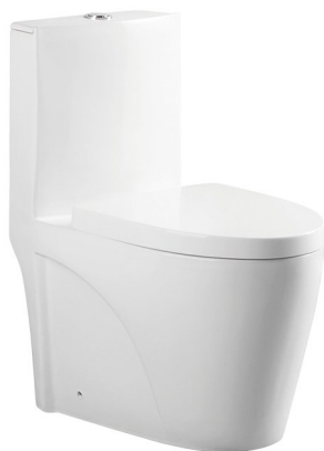
DA8001 虹吸/直冲连体坐便器 Siphonic/Washdown One-piece Toilet Size:750x390x775mm S-trap,250,300,400mm Roughing-in 地排污口中心离墙250,300,400mm P-trap,180mm Roughing-in 横排污口中心离地180mm
