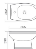
DF004 妇洗器 Bidet Size:565x362x390mm Fixing to wall with back 背靠墙式安装
