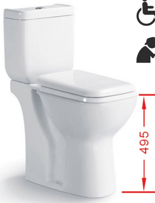
DT8040H 直冲分体坐便器 Washdown Close-couched Closet Size:670x370x880mm S-trap,220,250mm Roughing-in 地排污口中心离墙220,250mm P-trap,180mm Roughing-in 横排污口中心离地180mm
