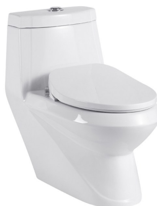
DA8061 虹吸/直冲连体坐便器 Siphonic/Washdown One-piece Toilet Size:705x370x790mm S-trap,250,300,400mm Roughing-in 地排污口中心离墙250,300,400mm P-trap,180mm Roughing-in 横排污口中心离地180mm
