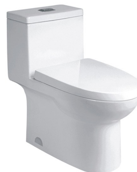
DA8324 虹吸连体坐便器 UPC Siphonic One-piece Toilet Size:685x380x705mm S-trap,300,400mm Roughing-in 地排污口中心离墙300,400mm
