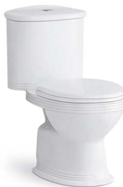
DT2004 直冲分体坐便器 Washdown Close-couched Closet Size:685x405x790mm S-trap,250,300mm Roughing-in 地排污口中心离墙250,300mm P-trap,180mm Roughing-in 横排污口中心离地180mm
