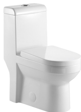
DA8061 虹吸/直冲连体坐便器 Siphonic/Washdown One-piece Toilet Size:705x370x790mm S-trap,250,300,400mm Roughing-in 地排污口中心离墙250,300,400mm P-trap,180mm Roughing-in 横排污口中心离地180mm
