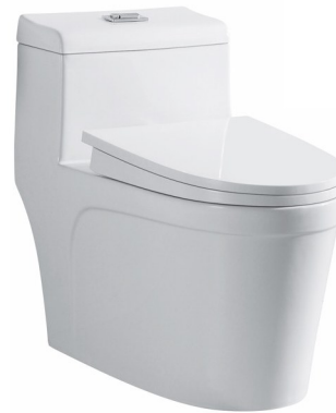
DA8075 虹吸/直冲连体坐便器 Siphonic/Washdown One-piece Toilet Size: 725x400x650mm S-trap, 250, 300, 400mm Roughing-in 地排污口中心离墙250, 300, 400mm P-trap, 180mm Roughing-in 横排污口中心离地180mm
