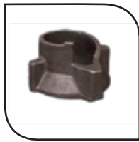
Malleable Cast Iron Top Cup Applicable on tube size: 48mm Dia Component Weight : 425 grams Surface Finish: Self Finished Application: Cuploc Scaffold system component used to tighten the horizontal Ledger
