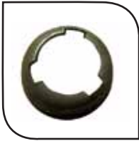
Pressed Sheet Metal Bottom Cup Applicable on tube size : 48 mm Dia Component Weight : 200 grms Surface Finish: Self finished Application: Cuplock Scaffold system component welded at the vertical pipe to hoist horizontal (pipe) Ledger
