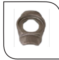
Drop Forged Ledger Blade End Applicable on tube size: 48mm Dia Component Weight : 210-215 grams Surface Finish: Self Finished welded at the end of horizontal (pipe) Ledger
