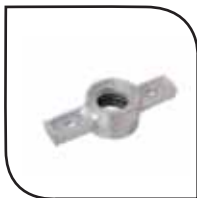
Pressed Sheet Metal Bottom Cup Applicable on tube size : 48 mm Dia Component Weight : 200 grms Surface Finish: Self finished Application: Cuplock Scaffold system component welded at the vertical pipe to hoist horizontal (pipe) Ledger
