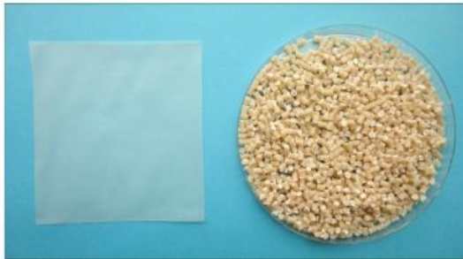
Figure 1. Visual presentation of the test item (left: film sample – right: pellets).
