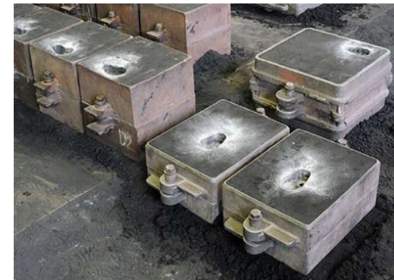
Sand Casting : Molding & pouring set-up with all accessories
