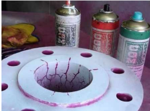
NDT- DP. testing set-up available
