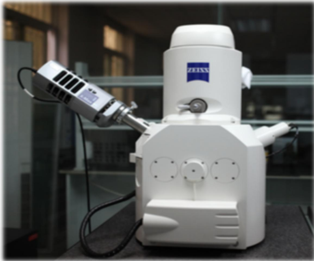
Instrument brand: Zeiss Tungsten filament scanning electron microscope Instrument model: EVO-18
