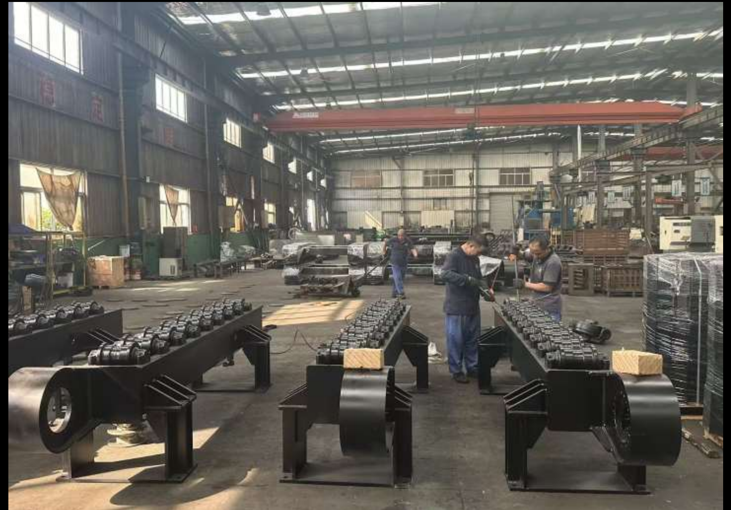
安装支重轮 ( Workers are installing track rollers )
