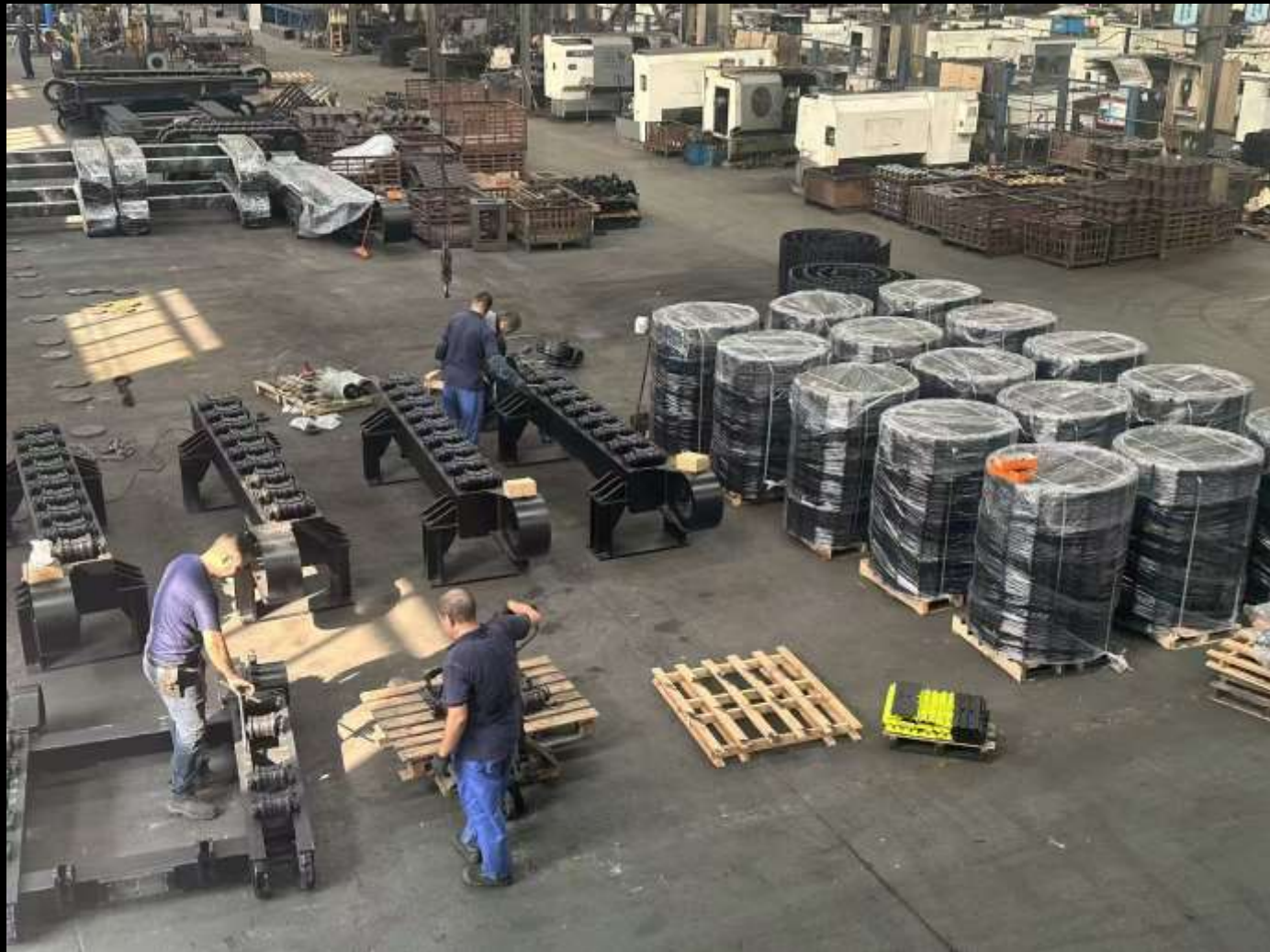
安装支重轮 ( Workers are installing track rollers )
