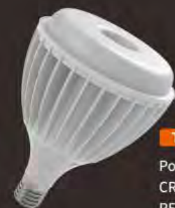
TB02-T170 Power: 150W CRI: >80 PF: ≥0.5/0.9 Input: 100-240V Base: E27/E40
